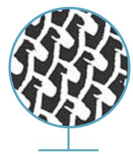
Monofilament Mesh is a woven fabric where each thread is a single filament, boasting excellent strength with no fiber migration. Providing extra strength and abrasion resistance, and offering a broad range of chemical compatibility, Monofilament Mesh bags are available in nylon, polyester and polypropylene.
