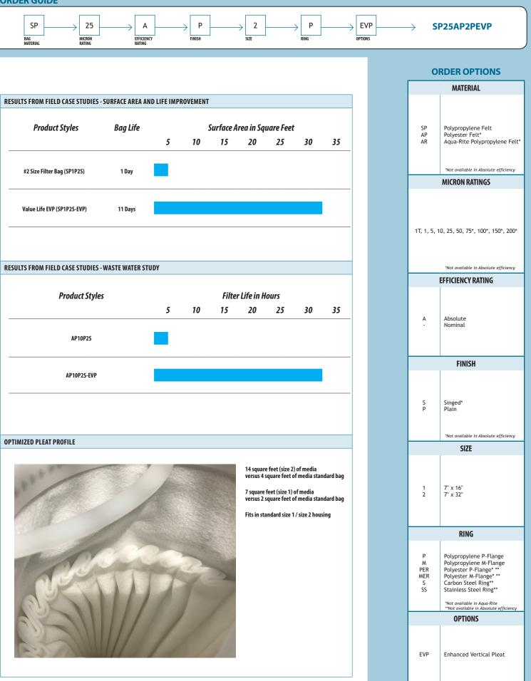
Strainrite's EVP (Enhanced Vertical Pleat) filters are the product of years of successful, application specific filtration in a variety of industries, using the Model 8T as the genesis of the Value-Life Series.
