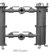
The SRID Duplex filter systems offer great flexibility for continuous on-line filtration requirements. This allows for continuous operation by directing the flow from one vessel to another by opening and closing of valves. This allows one side to be serviced, while the other vessel is in use.
