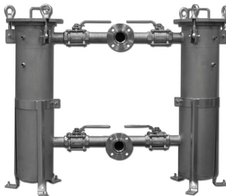
The **SRID Duplex** filter systems offer great flexibility for continuous on-line filtration requirements. This allows for continuous operation by directing the flow from one vessel to another by opening and closing of valves. This allows one side to be serviced, while the other vessel is in use.
